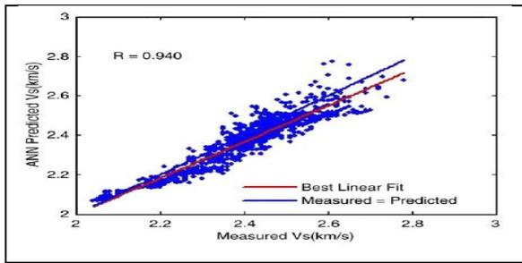
Figure. 3: Shear wave velocity prediction by use of ANN (Artificial Neural Network) [12].
