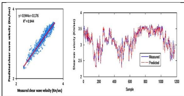
Figure. 5: Shear wave velocity prediction by use of SVR (Support Vector Regression) [9].
