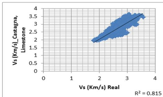
Figure 15: Comparison of real versus predicted shear wave velocity from Eq 10 values in well B.
