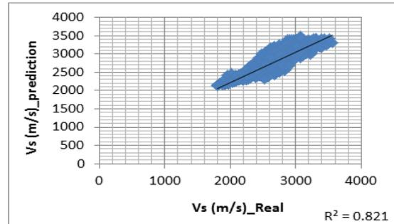
Figure. 8: Comparison of real versus predicted shear wave velocity from Eq 17 values in well B.
