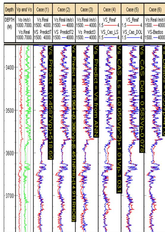
Figure 18: Real and predicted values of shear wave velocity in well B (3348m-3787m). For cases 4 and 5 V in km/s.
