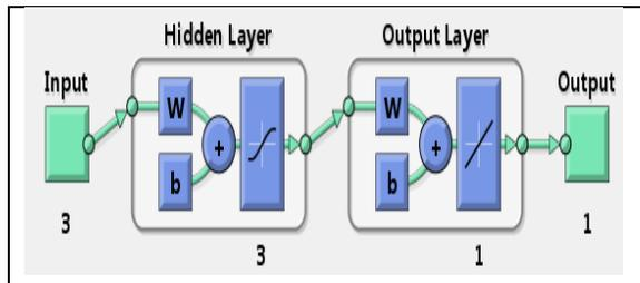
Figure. 12: Schematic of constructed network to shear wave velocity prediction.
