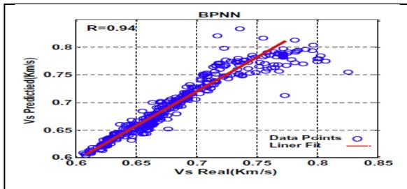
Figure. 4: Shear wave velocity prediction by use of BPNN (Back Propagation Neural Network) [11].
