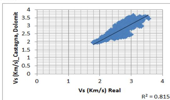
Figure 16: Comparison of real versus predicted shear wave velocity from Eq 11 values in well B.
