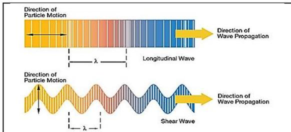
Figure. 2: Schematic of shear wave and compressional wave propagation direction. [6]
