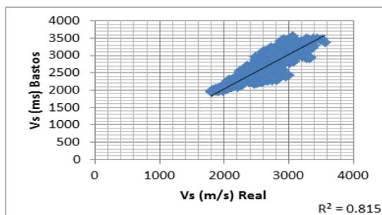
Figure 17: Comparison of real and predicted shear wave velocity from Eq 12 values in well B.
