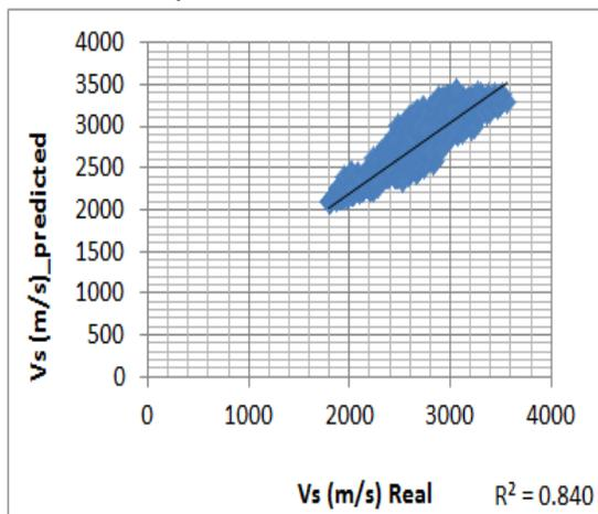
Figure. 11: Comparison of real versus predicted shear wave velocity from Eq 18 values in well B.
