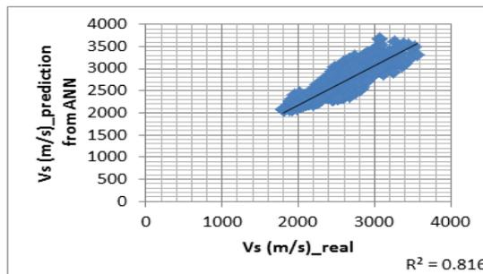
Figure. 14: Comparison of real versus predicted shear wave velocity from ANN tool values in well B.
