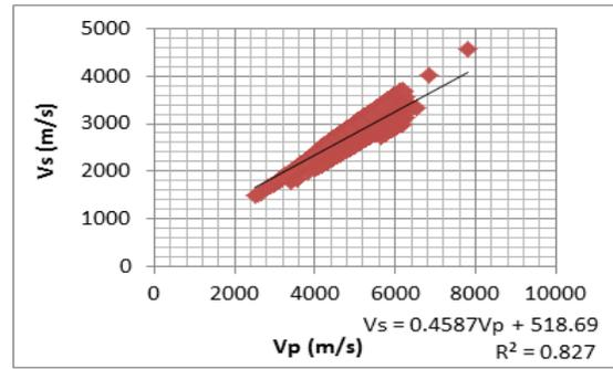
Figure. 7:  $V_p$  versus  $V_s$  in well A.
