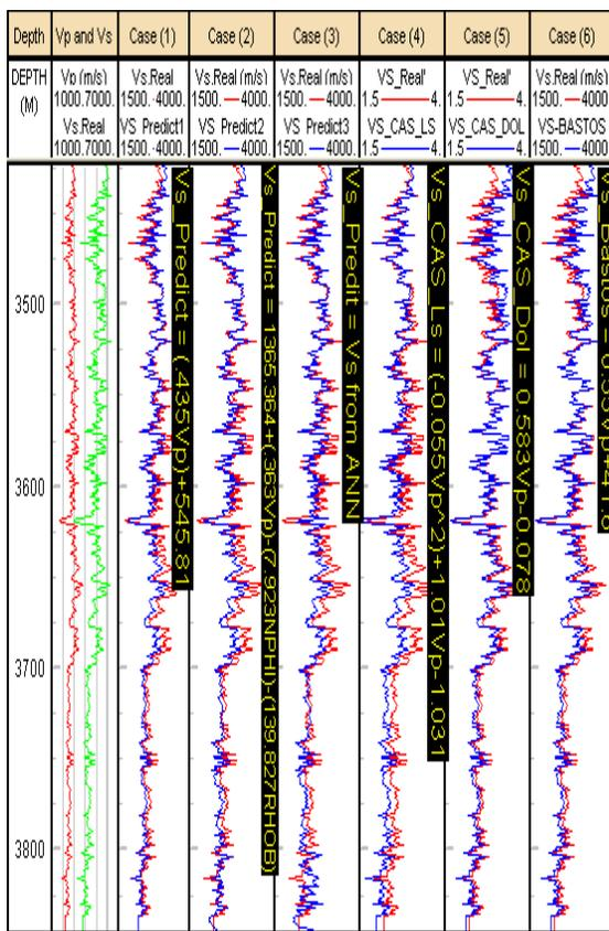
**Figure. 19: Real and predicted values of shear wave velocity in well A (3420m-3844m).**
